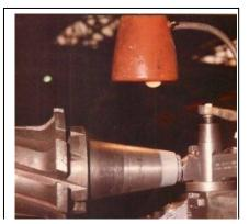
Shaft Repair with E.M.P. Inc. SUPERGRADE METAL, application, cure & lathing. In-Situ shaft repairs can also be made with Supergrade.
