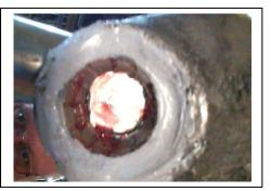
Bearing Housing Repair conducted on a tractor bucket loader, wheel rotator, bottom bearing hinge assembly. Void was egg shaped. E.M.P. Inc. SUPERGRADE METAL was installed, metal rebuilt and void brought back to original.
