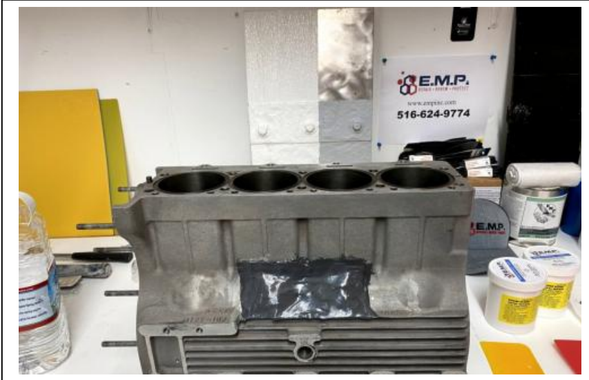
Fig 5. a) Brush thin coat b) apply epoxy c) install Fiberzite fabric d) apply Engine Block Repair Epoxy again as per product spec.
