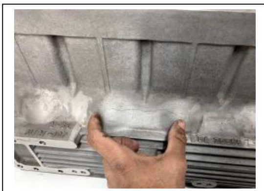
Fig 1. Crack in water jacket about 4"-5".
