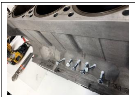
Fig 3. Bolts inserted through the crack.
